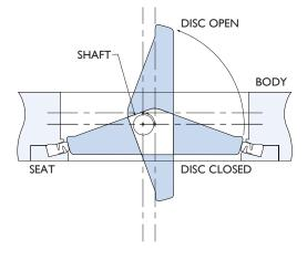
The double offset shaft design assures bi-directional sealing throughout the full pressure range of the valve. The cam-like action produced by the offset disc effectively lifts the disc off the seat during the initial opening of the valve thus reducing seat wear and eliminating seat deformation. When the disc is in the open position no contact exists with the valve seat. This effectively reduces operating torques while extending seat life.
