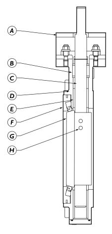
**Bushings** High temperature fiberglass composite backed RPTFE ensuring maximum shaft support.
