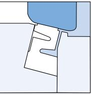
Disc in closed position; Line pressure applied from right side.
