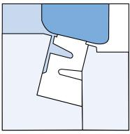
Disc in closed position; Line pressure applied from left side.
