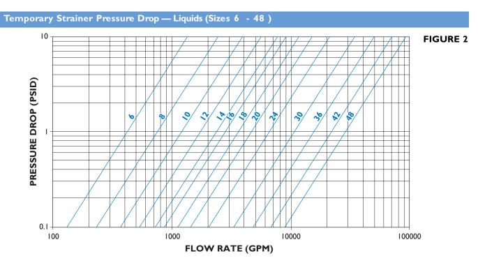
Notes: I. Pressure drop curves are based on water flow with standard screens. See page 28 for correction factors to be used with other fluids and/or screen openings.
